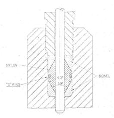
The packing gland. Nylon was chosen as the packing material because it provided sealing with minimum frictional losses
